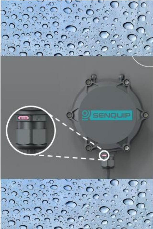
If enclosures are not equipped with pressure compensation vents, heating and cooling cycles can result in moisture being drawn into the enclosure. The effect is worse with a better sealed enclosure as water is drawn up through the wiring loom. Not only are the electronics in the enclosure damaged, but the wiring may be corroded. The effect is often seen on trailers with sealed lights. As the lights are turned on and off, each time the lights cool, moisture is drawn up the wiring loom.
